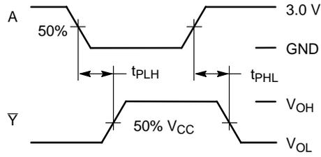
**Figure 4. Switching Waveforms**
