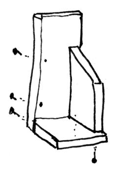
Rough guide for positioning & screws size 5 x 50
