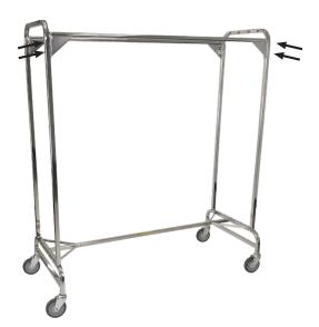
**Model 722/725:** Position one upper crossbar as pictured, with flush side of triangular support facing out. Align crossbar and upright holes and secure with two partial-thread bolts on each side, with nuts on the side of triangular support. Repeat for other crossbar.
