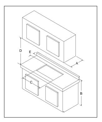
NOTE: Do not install closer than 1/2 inch (12 mm) from any adjacent surface.
