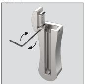
Tighten the hinge pin screw with a 1.5mm Hex Key by turning clockwise. The lid should rotate freely.
