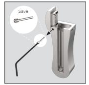
Remove the hinge pin screw and set aside, it will be reused to install the new lid.
