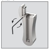
Loosen the hinge pin screw using a 1.5mm Hex Key (Allen Wrench) and turning the screw counterclockwise.
