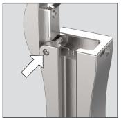
Locate the hinge pin screw on the upper left side of the bracket.
