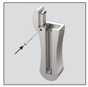
Carefully align the locking lid assembly and reinstall the hinge pin screw by gently pushing it through the bracket and new locking lid assembly.
