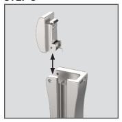
Remove the old locking lid assembly by lifting straight off.
