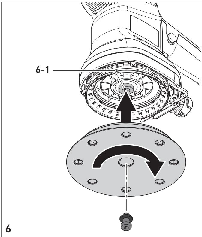
The grinding disks and the tool-holding fixture on the appliance are equipped with a positive holder **[6-1]**.
