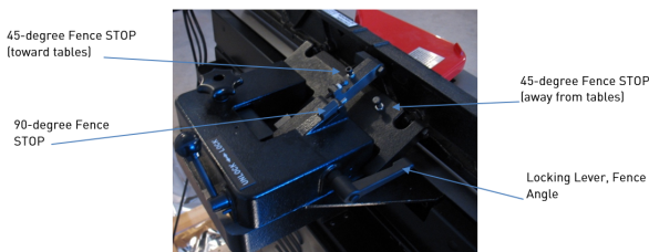
FIGURE 16: FENCE ANGLE ADJUSTMENT COMPONENTS
