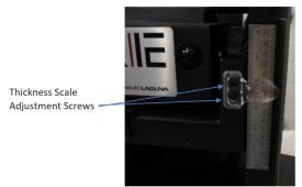
Figure 7: Thickness Scale Calibration
