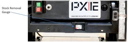
Figure 9: Stock Removal Gauge
