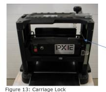
Carriage Lock "UP" Unlocked "DOWN" Locked
