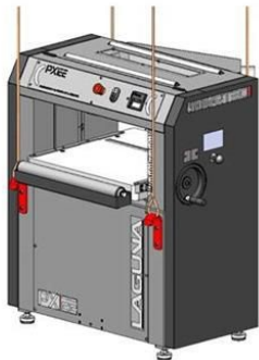
FIGURE 1: LIFTING PLANER WITH HOOKS AND HARNESS
