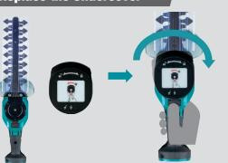
Place the undercover by lining the  $\square^{\cap}$  with the  $\blacktriangle$  on the tool. Confirm that the lock lever is in the groove of the undercover. Then, while pressing the undercover in, turn the undercover clockwise until the  $\square$  aligns with the  $\blacktriangle$  on the tool.
