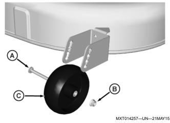
42A Mowers - Remove carriage bolt (A) and nut (B). Move wheel (C) to desired hole position. Install wheel to deck with carriage bolt and nut. Tighten nut to specifications.
