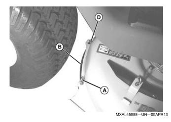
4. Install right mower deck gate (B) onto slotted hole (D) on bottom of mower deck, and secure opposite end
