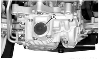
a. Remove cap (E) from front side of transmission using a 3/8 in. ratchet.
