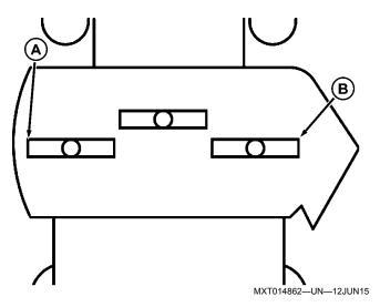
b. Turn left blade (A) as shown. Hold drive belt and turn right blade (B) as shown. Take measurement for both blades.
