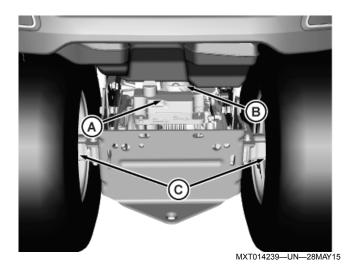
4. On or near transmission (A), transmission fan (B), and driveline (C).
