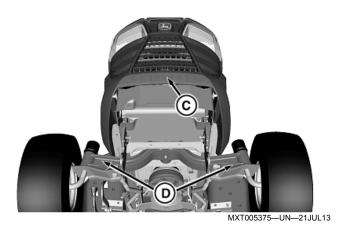
Safely lift front of machine at machine frame point (C). Place jack stands or other stable supports onto front axle locations (D). Block back wheels if only lifting front of machine. 4. To lower machine, lift front and/or rear of machine, and remove jack stands or supports. Lower machine.
