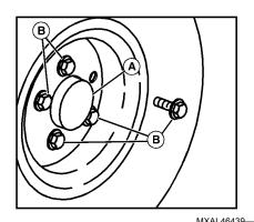
MXAL46439—UN—05APR13 Wheel may or may not have a cap (A) to remove when removing the wheel.
