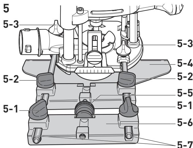
*This distance can be adjusted faster and more precisely with the fine precision adjustment [5-6] available as an accessory:*
