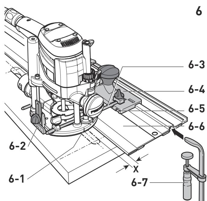
When working with marking-up lines, the marks on the platen [6-1] and the scale on the support [6-2] show the centre axis of the cutter.
