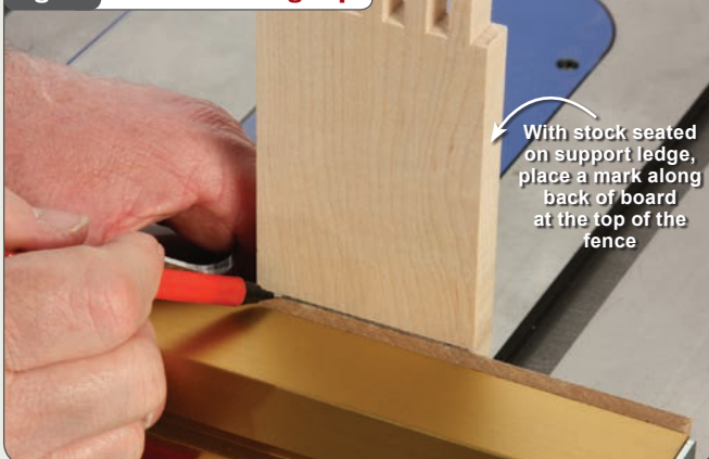
Fig. 30 Stock Marking Tip
