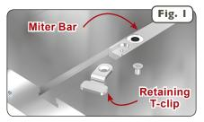
Using the supplied 3/32" hex key, adjust each of the (3) visible miter bar expansion disks for a zero-side play, sliding fit in your miter channel as shown in Figure 2. Turning the fastener clockwise EXPANDS the bar width. The disks are designed to require a fair amount of adjustment torque for proper expansion.
