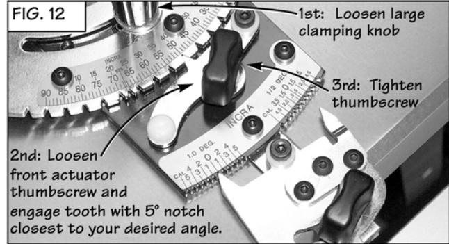
**2** Loosen the rear actuator thumbscrew. Use the left-hand tooth to add or subtract from the coarse adjustment setting in  $1^\circ$  intervals. Use the right-hand tooth to add or subtract from the coarse adjustment setting in  $1/2^\circ$  increments. Engage the tooth firmly in the selected notch, then tighten the large clamping knob and the rear actuator thumbscrew, Fig. 13. **Important:** After completing your cut, don't forget to return the rear actuator setting to the  $0^\circ$  notch.
