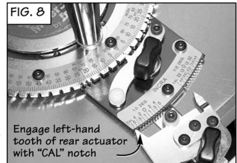
Now pivot the rear actuator to engage the right-hand tooth with the notch marked "CAL" on the rear scale, Fig. 9. If adjusted properly, it will pivot perfectly into the notch. To adjust, loosen the (3) socket head screws that secure the tooth and fine-tune the position to align with the "CAL" notch. Pivot back and forth between the two "CAL" notches to verify the calibration.
