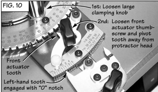
**2** Rotate the protractor head to the desired angle, then firmly engage the tooth on the front actuator with the corresponding notch on the protractor head. The actuator tooth should point directly to the desired angle on the scale. Tighten the large clamping knob, then tighten the front actuator thumbscrew, Fig. 11.
