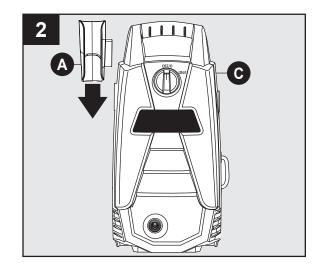
Slide spray gun holster (A) onto left side, when facing the power washer unit (C) as shown.
