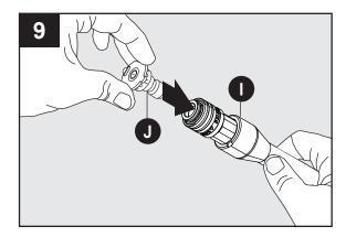
Attach nozzle (J) into end of lance (I) by pressing selected nozzle into place. It will make a "click" sound when firmly in place.
