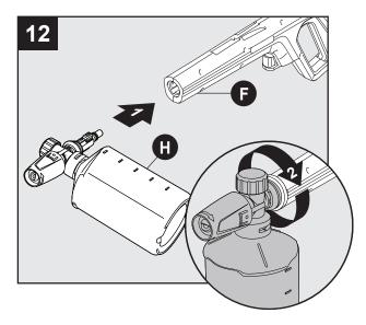
Insert foam cannon (H) into spray gun (F), push in and turn clockwise.
