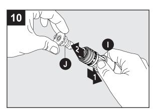
To remove nozzle (J) pull back on collar of lance (I) and pull out nozzle.
