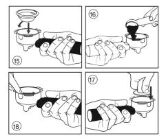
**IMPORTANT:** Be sure not to overfill the filter basket with coffee as this can cause the portafilter holder to leek or overflow
