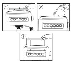
4. To fill the espresso machine with water, simply lift the lid of the water reservoir at the top of the espresso machine, (1) and fill with fresh cold water or filtered water (2) or remove the reservoir and place the water reservoir down firmly until the reservoir cover is flush with the top of the espresso machine (3).
