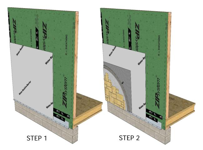
Pro Tip: The building science industry promotes the use of a drainage gap behind porous claddings like adhered stone.
