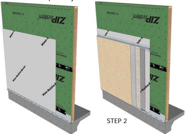
Pro Tip: The building science industry promotes the use of a drainage gap behind porous claddings like stucco.
