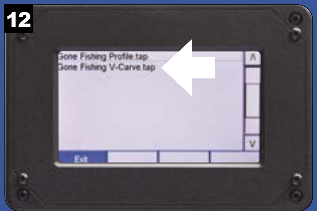
12 From the list of available projects, select your chose .tap file to proceed.
