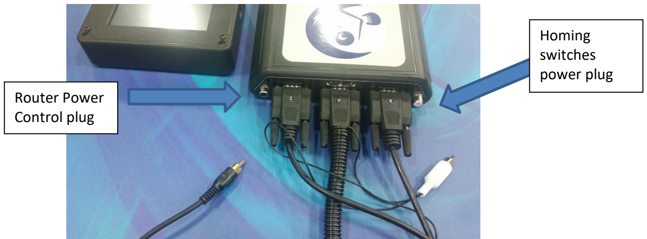
Attaching cables to the back of the Shark SD120 controller
