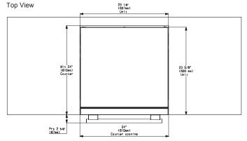
Thermador Double Drawer under counter top dimension. (Unit door flush with cutout)
