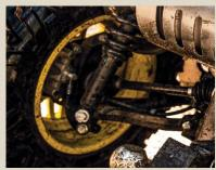
High-strength cast-iron knuckle and upper A-arm support the high stresses of the shocks, constant-velocity (CV) shaft, and wheels in rocky terrain.
