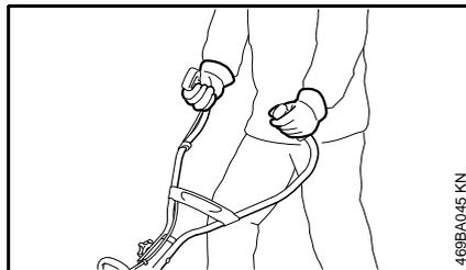
Always hold the unit firmly with both hands on the handles while you are working. Wrap your fingers and thumbs around the handles, keeping the handles cradled between your thumb and forefinger. Keep your hands in this position to have your power tool under control at all times.
