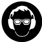
To reduce the risk of injury to your eyes never operate your power tool unless wearing goggles or properly fitted protective glasses with adequate top and side protection complying with ANSI Z87 "+" (or your applicable national standard).
