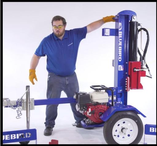
Use handle at top to lower the boom and secure the pin, see pictures below.
