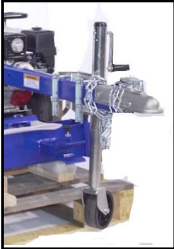
Rotate the jack to upright position and lower the wheel so the tongue will be level when installed.
