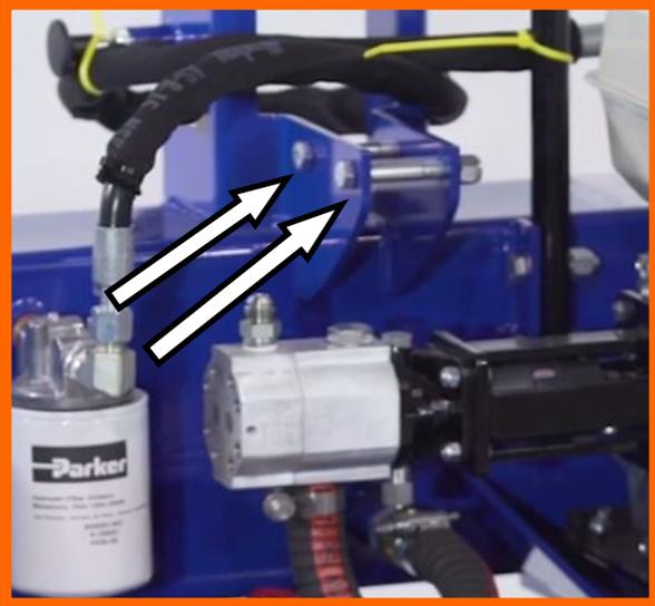
Remove these two bolts , they will be used for attaching the tongue.
