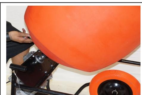
**Step 8** — Attach the Bushing & Flange (with drum attached) to the motor. Line up pre-holes on the Bushing & Flange to the Shaft.
