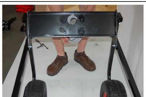
**Step 4 -**Install gear motor, as shown.
