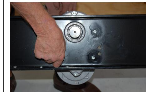
**Step 5 –** Tighten by first installing the flat washers, the lock washer, then the nuts on all 4 studs. Tighten to 10 pounds of torque.
