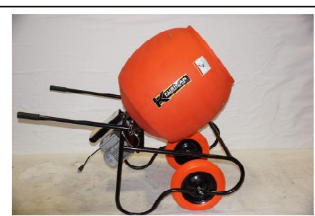
**Step 11** — Install handles from front to back and secure with lock pins that are attached to the frame. Install grips and you are done.
