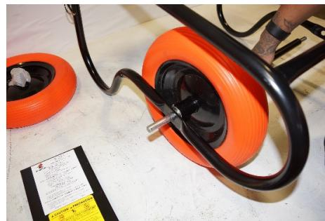
**Step 2—**place wheels inside the frame with long end out. Insert Wheelbarrow Axle through the frame into the tire and through the Axle Tube Spacer, then through the other tire. Once in place insert the 5/8" steel washer and the "R" Clip at the ends of the Wheelbarrow Axle.
