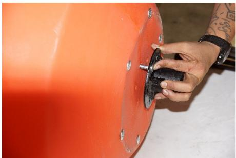
**Step 6** — Attach the Bushing & Flange to the back of the drum using the Whizlock Screw 3/8" x 1-1/2".
