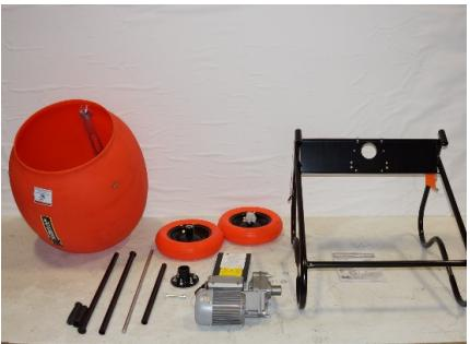
**Step 1-** Remove all the shrink wrap from parts. Layout all part to identify each one.
