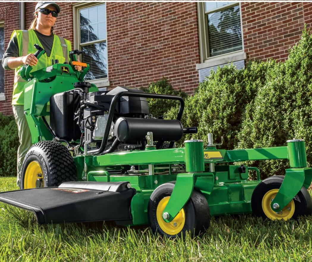
The M and R Series both feature a thoughtful design that promotes safe operation. Before the engine will start, the transmission speed lever must be in neutral, the parking brake set, the PTO disengaged and the key switch turned to on.
