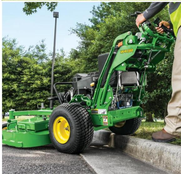
And for sheer curb climbing ability, our four R Series walk behinds are built with 8 and a half inches (21.6 cm) of frame clearance and positive reverse performance bringing even the most daunting curbs to their knees. No more scuffed or chipped curbs. And no more damage to the mower.
