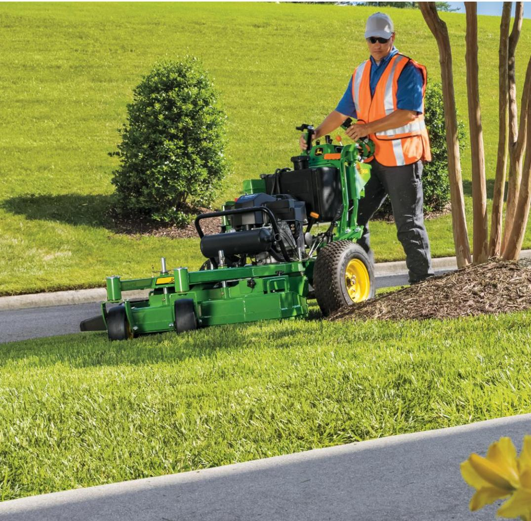
Both the M and R Series feature engines with a V-Twin design for smooth operation and fast starts. The aluminum engine block with cast-iron cylinder liners dissipates heat quickly. And the overhead valve design has:
