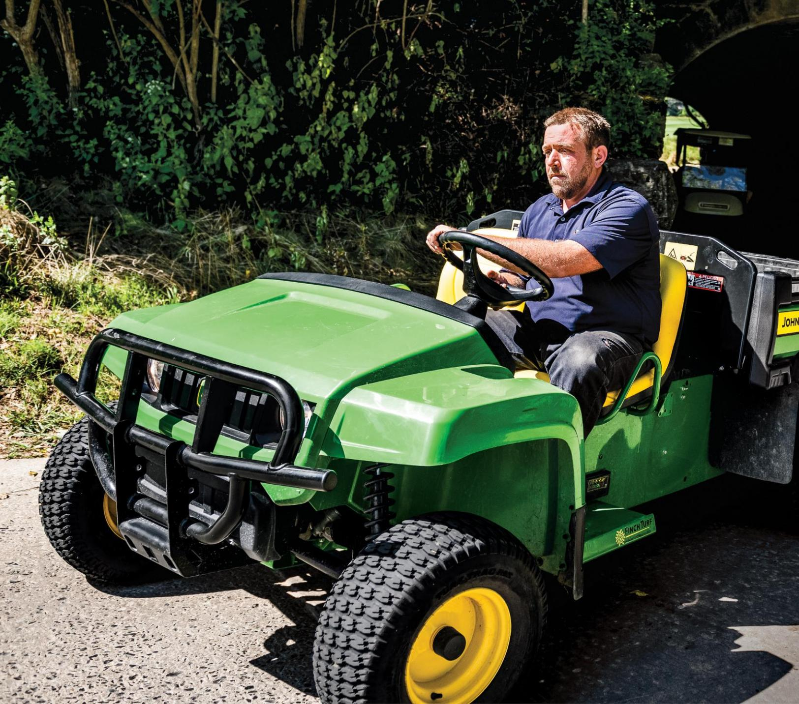
The 48-volt electrical system performs steady and smooth all day long.\* This transporter with zero operating emissions sports a 16.4 cubic foot (.46 cu m) capacity reinforced cargo box, the ideal solution for working inside large warehouses and buildings. The pick-up style tailgate and tie-down points make managing loads easier. For large loads, convert to flatbed mode by removing tailgate and side panels.
