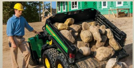
**A standard gas assist shock** underneath the bed makes lifting and dumping effortless. An optional power lift kit raises and lowers bed from a switch right on the dash.
