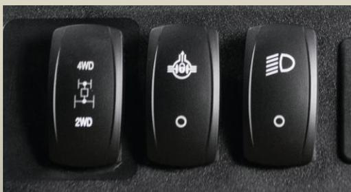
4WD instant engagement provides traction with a flip of a switch. Auto-locking electronic differential button provides a more automotive feel for instant engagement at your fingertips.
