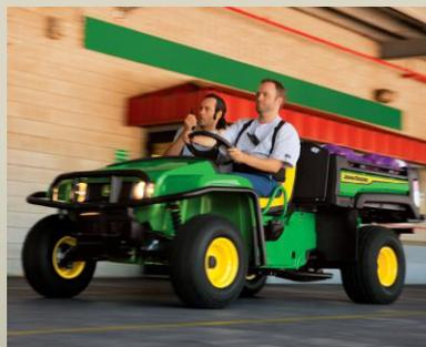
No matter what you haul, the Gator™ TX delivers a smooth ride, courtesy of its four-wheel suspension with coil over shock, triple-rate adjustable springs.
