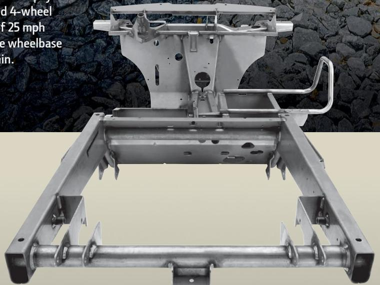
The hydroformed frame on the HPX has incredible tolerance for twisting and heavy loads.
