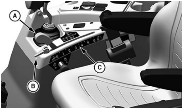
A—Rockshaft Control Lever B—Rockshaft Depth Stop C—Rockshaft Position Identifiers
