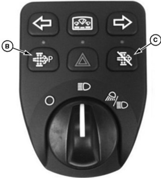
LV17595—UN—21MAY13 Exhaust Filter Cleaning Mode Switch
