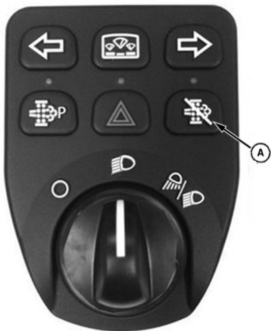
LV26014—UN—24AUG16 Exhaust Filter Cleaning Disable Switch
