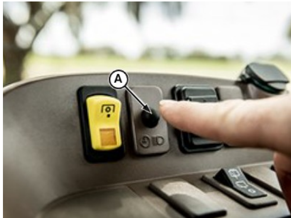
A—Go Home Lighting Switch B—Headlights (2 used)
