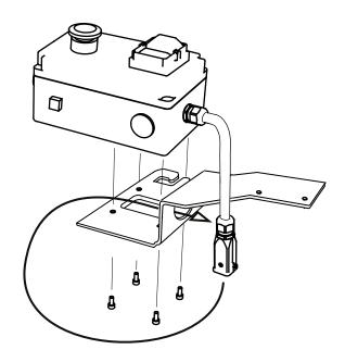
To install the crank handle on the electric saw, you first remove the existing handle and then fit the crank handle using the existing hole pattern and the original bolts. Assemble in the following order: handle, mount+elelctrical box, saw carriage and the crank under the saw carriage.
