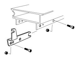
If the sawmill is equipped with a support leg, the smaller hole has to be used together with an Allen bolt M6X20.
