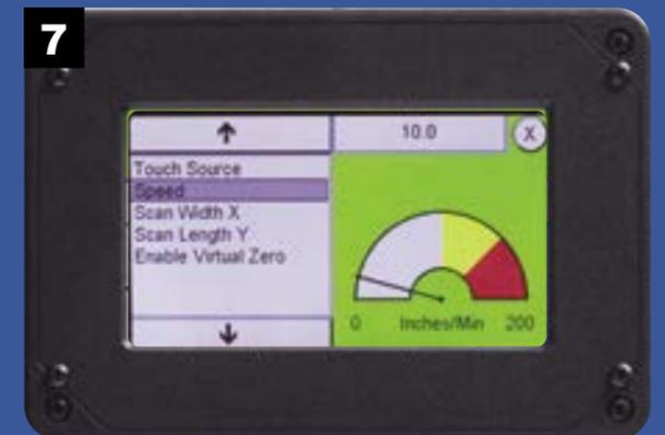
The Speed setting controls the Z-axis plunge rate. The default setting of 10 works well for most situations. Change it by pressing the settings field in the upper right and enter a new value using the numeric keypad.
