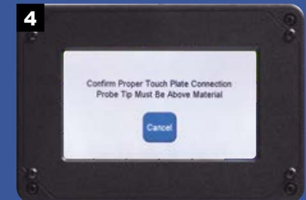
Raise the touch plate until it touches the router bit to confirm a proper connection.
