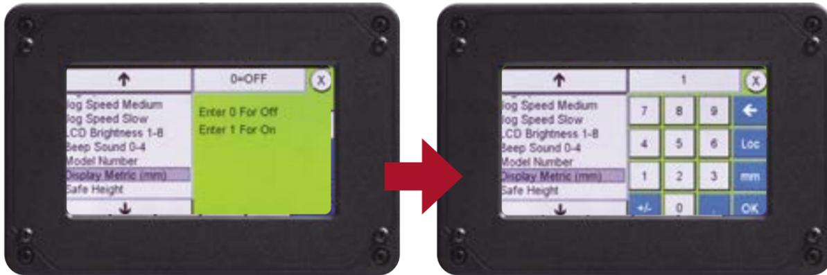
**Display Metric:** Toggles between millimeter and inch values displayed in the position fields on the main screen. Enter either 1 for metric or 0 for inches.
