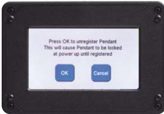
**Unregister LCD:** This option removes the access code from the Pendant.
