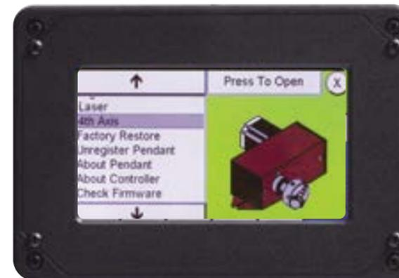
**4th Axis:** This app provides setup options for the various rotary 4th axis accessories available from Next Wave CNC. See the 4th Axis Owner's Manual for complete use and operating instructions)
