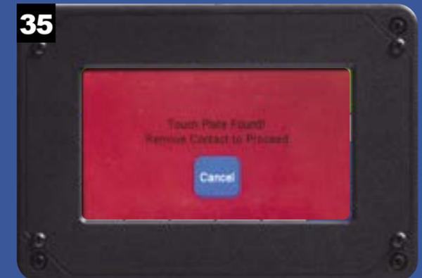
This screen confirms the touch plate is connected properly.
