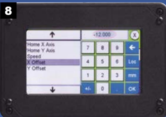
Enter a value to set the offset distance of the X-axis from 0,0. Repeat the process to set the Y Offset.
