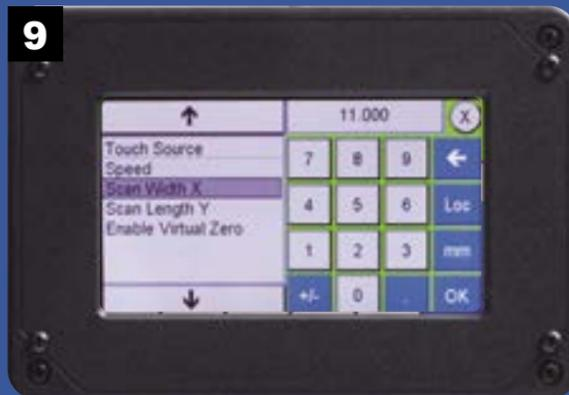
After choosing "Scan Width X," enter the width in the upper right hand field using the numeric keypad, then press OK to continue.
