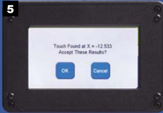
Press OK to accept the X-axis location. Repeat the process to calibrate the Y-axis.
