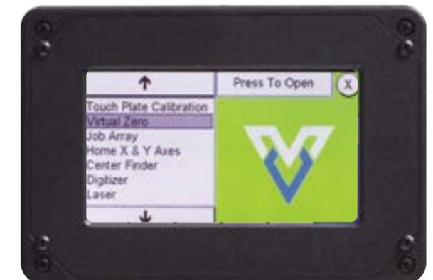
**Virtual Zero:** Select this app to adjust the .tap cutting file to conform to a slightly warped, curved, or uneven project material or machine table (see next page).
