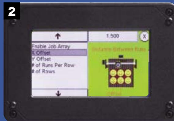
The X and Y Offsets sets the distance between the XY datum points for each copy of the part defined in the design file. Enter the distance in the upper right field using the keypad.
