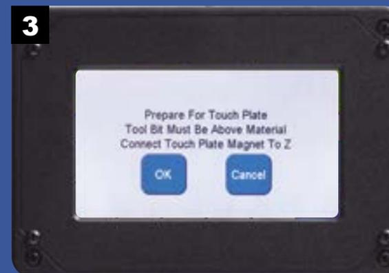
Make sure the magnet is attached to the router bit before pressing OK.
