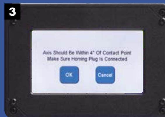
Make sure the router bit is within 4" of the lower left corner in the X- and Y-directions.
