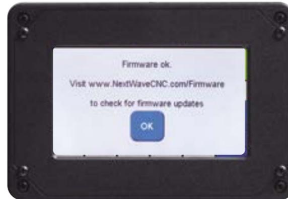
**Check Firmware:** This app runs a quick check and displays a status report on your firmware. Firmware updates are available at [NextWaveCNC.com](http://NextWaveCNC.com).
