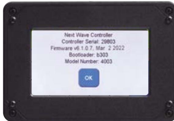
**About Controller:** This displays the controller (control box) serial number and firmware information.
