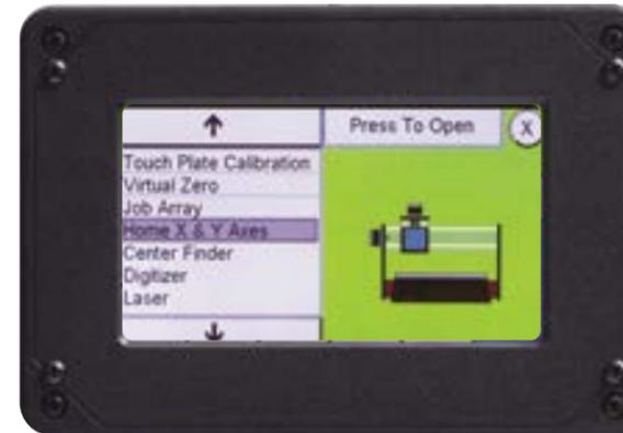
**Home X & Y Axes:** This app calibrates and zeroes out the X- and Y-axes to the machine's home location in the lower left corner of the table (page 15).
