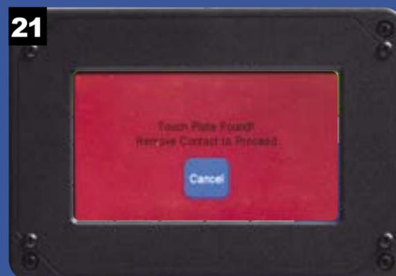
When you touch the plate to the router bit, the red confirmation screen appears.
