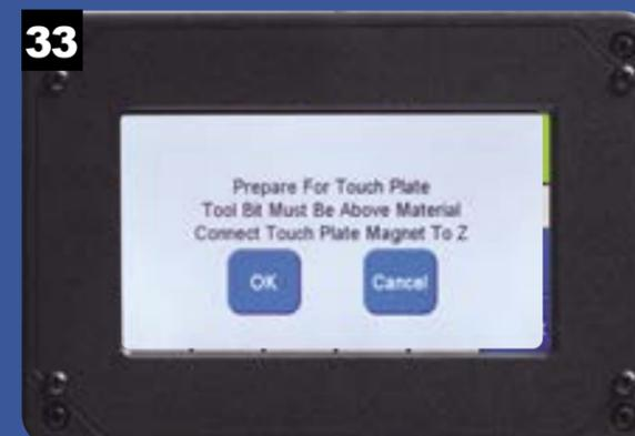
Ensure the touch plate is positioned directly below the router bit and select OK.
