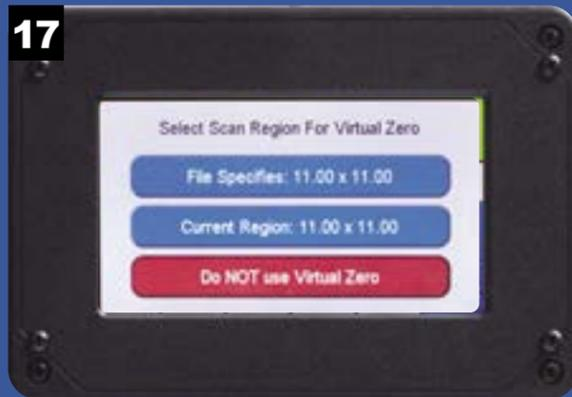
On this screen, you're presented with two options. The first, File Specifies, displays the material size you set up in VCarve less 1". This provides half of an inch clearance around the material to assure the scan area stays within the boundary of the material, and to allow some room for clamps.
