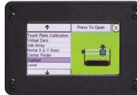
**Digitizer:** Use this app to map the shape of your project using the Digital Duplicator accessory. You can create a copy of an existing carving or use the scan data with the Virtual Zero app. See the Digitizer Owner's Manual for complete use and operating information.
