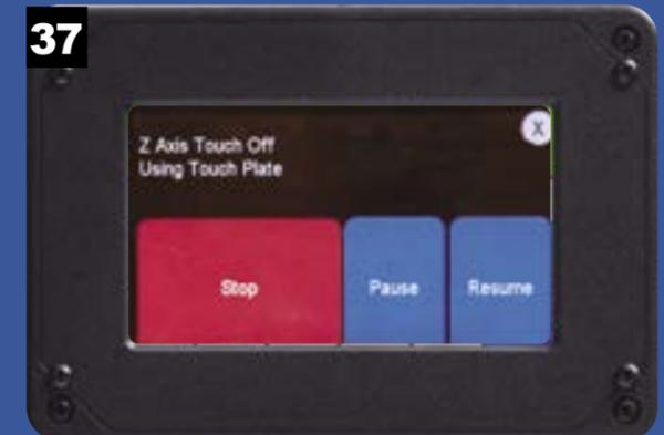
Allow the router to move down until it touches the plate.
