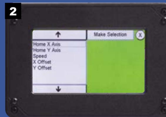
Select Home X-axis to calibrate the zero point for the X-axis home position.
