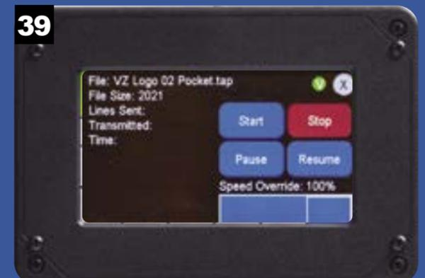
Press Start to begin processing the file. The Virtual Zero map can be used as many times as needed for your project. Remember that the mapping is specific to a particular piece of material, so if you install a new piece of material the mapping must be redone.
