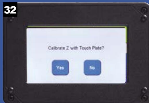
With a new router bit installed, you will need to recalibrate the bit's Z zero with the touch plate once again.
