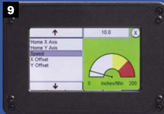
The Speed function allows you to set the speed the router moves to the Home position.
