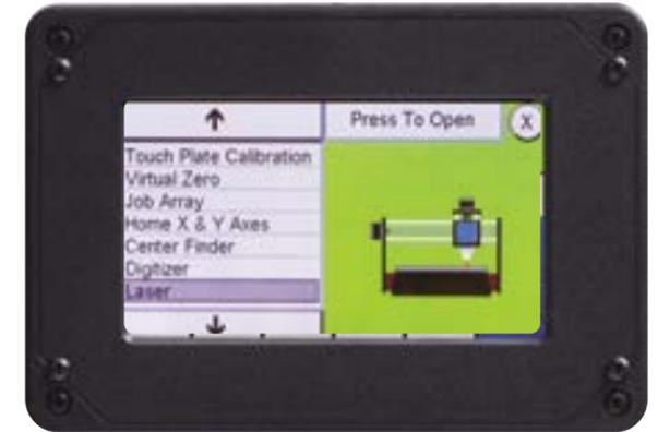
**Laser:** Use this app with the laser accessory to create detailed laser-engraved photographic engravings, images, and lettering. See the Laser Owner's Manual for complete use and operating instructions.
