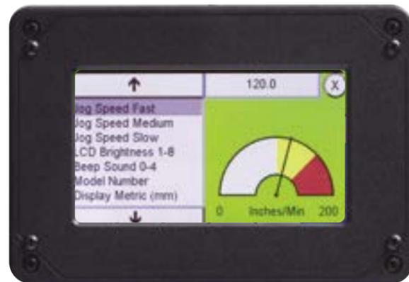
**Jog Speed:** Press Jog Speed Fast, Medium, or Slow to display the jog speed settings window. The current jog speed appears in the top right of the
