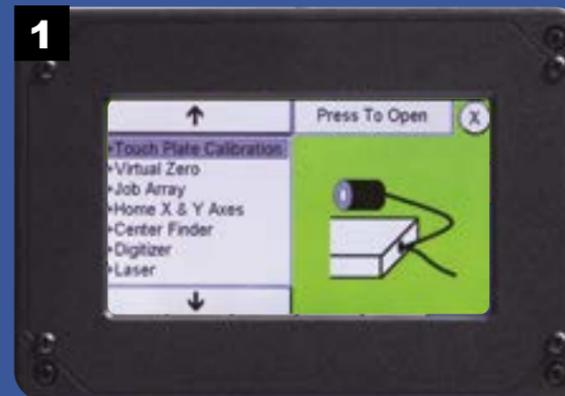
Press the APPS button on the Main screen to access the option to calibrate the touch plate.
