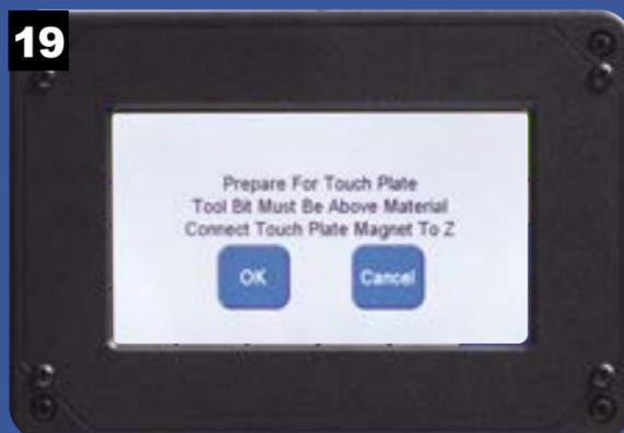
With the Z Zero Touch Plate connected to the Pendant, and its magnet attached to the router bit, press OK.
