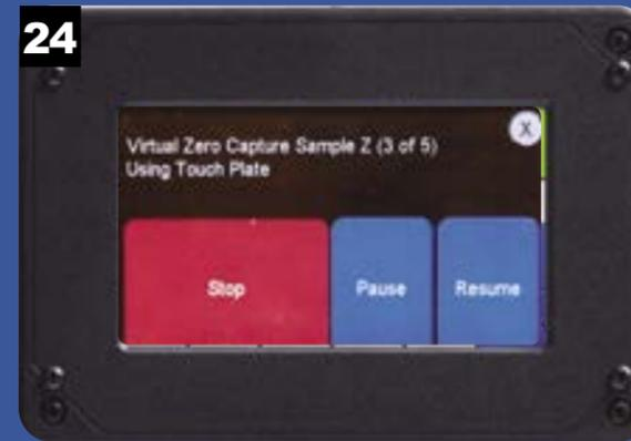
The router will move in the Z direction until it contacts the touch plate. Repeat the process to define all five points.
