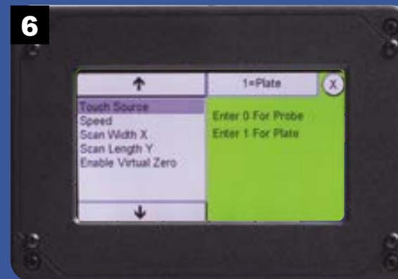
Press the field in the upper right of the screen to choose either the probe or touch plate using the numeric keypad. Enter 0 to use the probe or 1 to use the touch plate.
