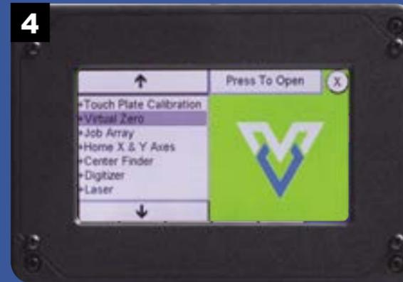
After inserting USB device, use the Apps key and select the Virtual Zero app. In the upper right of the screen touch Press to Open to display the Virtual Zero settings screen.
