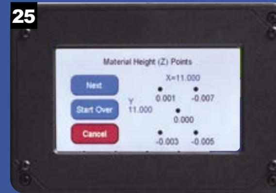
When the five Virtual Zero points are captured, the screen shows the X and Y values of the scan area and how much each capture point varies from the Z Zero height. Press Next to begin carving your project.
