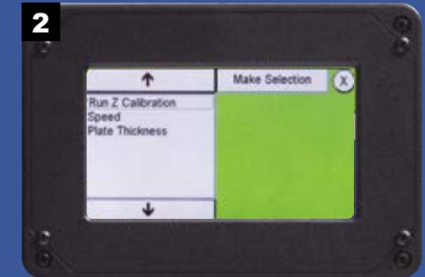
The Run Z Calibration option begins the routine to zero the Z-axis using the touch plate.
