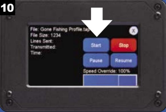
To begin the CNC operation, press the Start button. If needed, the Stop button shuts down the CNC.
