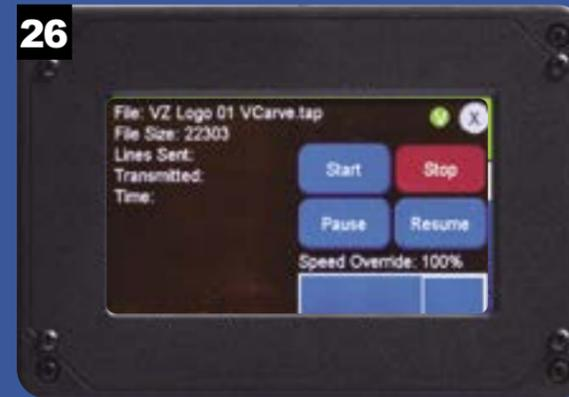
A small green V appears in the top right corner of the screen to signify that the file is using Virtual Zero. Press Start to begin carving.
