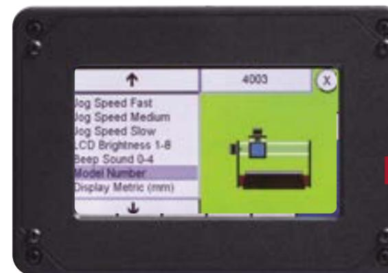
**Model Number:** This function controls several settings on your Shark CNC such as motor rotation and XY machine orientation. Verify the model number for your machine using the chart at right. Verify this setting after performing a firmware update for the Control Box or Pendant.
