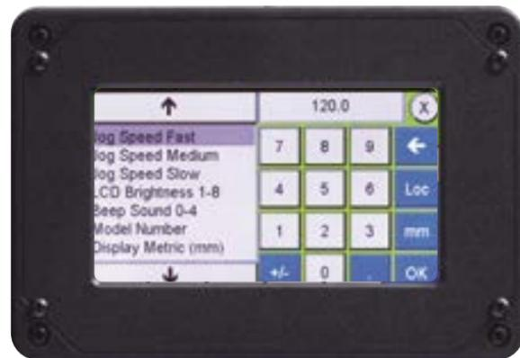
screen. Tapping this field opens a numeric keypad for entering a new value for the Jog Speed. Press OK to save the setting.
