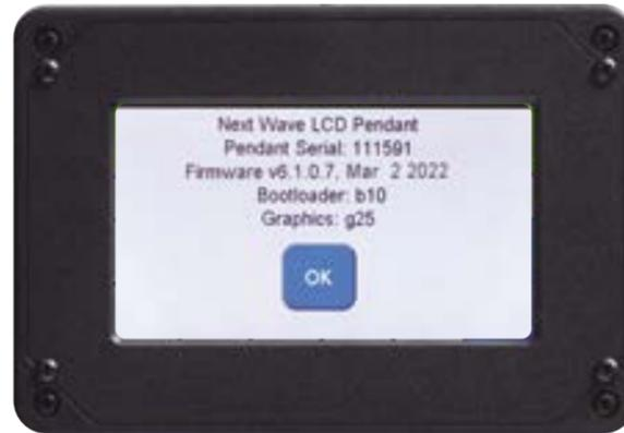
**About Pendant:** Use this to display the Pendant serial number and firmware information. This is useful to verify firmware versions or when communicating with technical support personnel.
