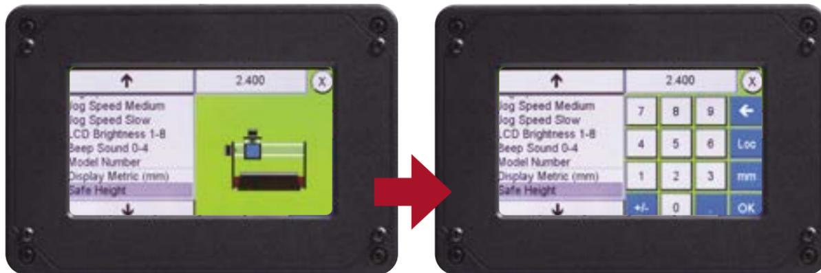
**Safe Height:** The Safe Z Height setting controls how far the router bit rises above the Z zero position when you press the Mv0,0 button on the Main screen. This function helps prevent router bit collisions and possible breakage with hold-down clamps or other hardware. You can adjust the Safe Height by pressing the Setup key on the Main Screen. Scroll down the list to "Safe Height" (Figure 1). Adjust the Safe Height by pressing the numerical field at the upper right of the screen. This
