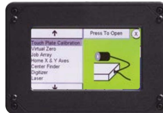
**Touch Plate Calibration:** Select this option then Press To Open to initiate a series of steps that quickly and accurately zeros out the Z-axis using the Z Zero Touch Plate accessory (see page 11) available from Next Wave CNC.
