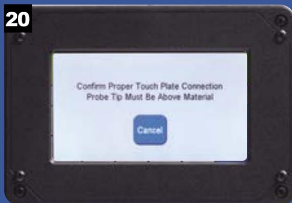
Confirm a proper connection between the plate and Pendant by touching the plate to the router bit.
