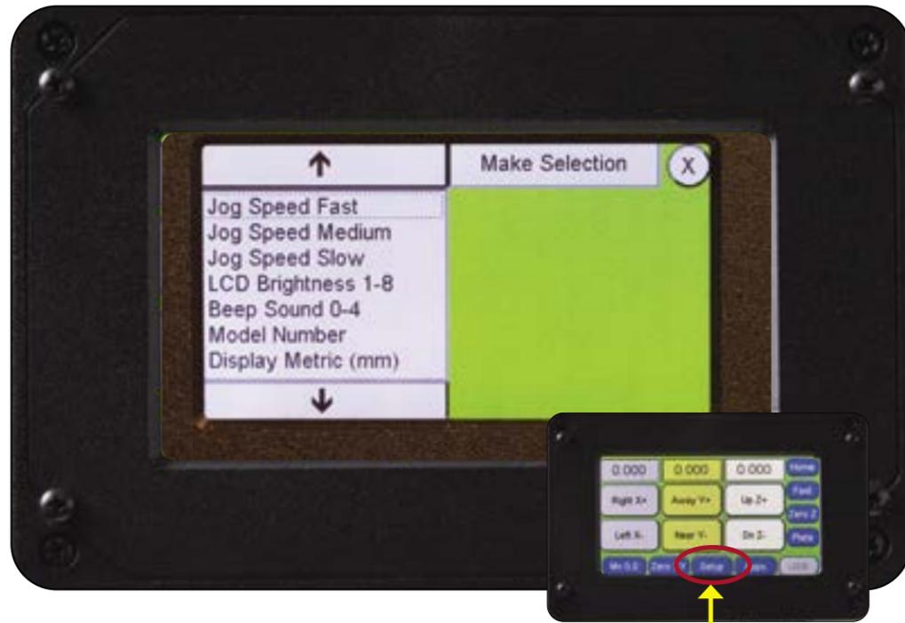
**Setup Menu Screen:** Press the Setup button on the Main Control screen to open the Setup screen. The Setup menu contains options for controlling specific Pendant functions. Press a menu item to open the settings screen for that option. To return to the Main Control Screen, press X in the upper right corner.
