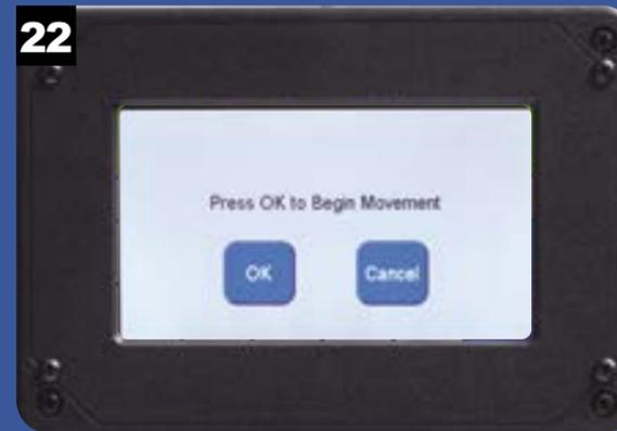
Ensure the touch plate is positioned below the router bit before continuing. Press OK to confirm that you're ready to capture Virtual Zero points. These are typically the four corners and center of the scan area defined earlier.
