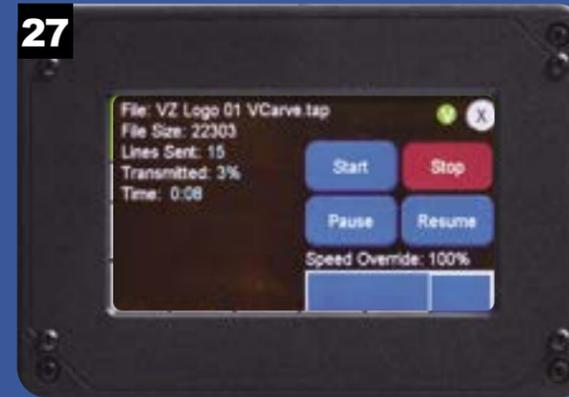
As the project file is being processed, the Lines Sent, Transmitted, and Time values are updated. After the first file is done running, press X to return to the main screen.
