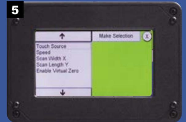
The Touch Source defines the method used to set the Z zero point. Many *Shark CNC* users will use the *Shark Z Zero Touch Plate*. You may also use the optional digital probe accessory.
