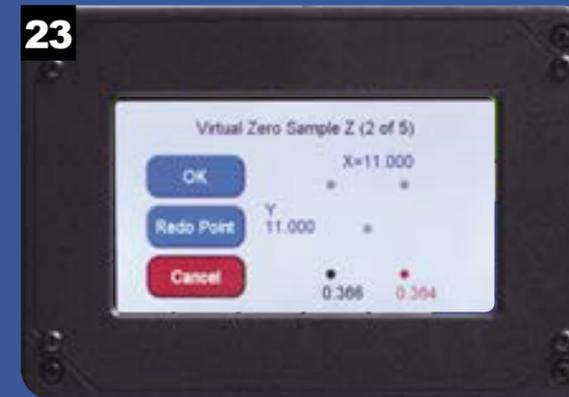
The Virtual Zero app records and shows how much each point varies from the original Z zero position. After scanning a point you can choose Redo Point or press OK to continue mapping.
