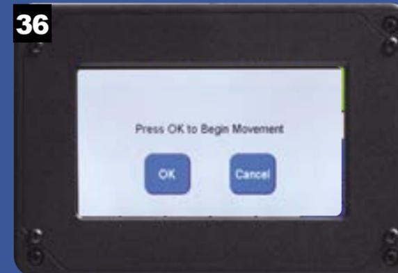
Place the touch plate below the router bit and select OK.
