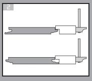
Pureplank 06 floors are designed for a floated installation. Do not use adhesive to bond the flooring to the subfloor or fix the flooring to the subfloor with nails or screws at any point. Never strike the boards directly with a hammer, always use the tapping block.
