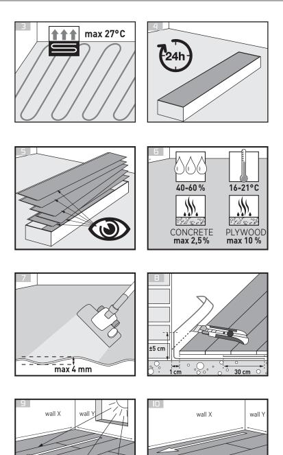
Pureplank 06 has an incorporated cork layer which performs the cushioning and sound-dampening functioning of an underlay. Where installing to a concrete or anhydrite screeded substrate, install Pureplank 06 over 250 micron polythene sheeting which should be laid at a 300mm overlaps and taped at joints with foil jointing tape. The polythene can continue 50mm on walls to ensure moisture venting from the substrate does not damage flooring.
