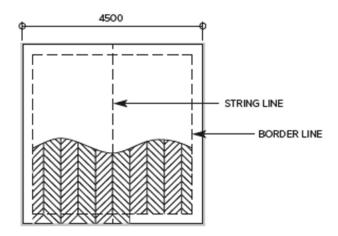
Versailles panel installations (and installations of other repeating elements) should be planned to ensure even cuts are present to all perimeter walls. Once the layout of the floor is established, either a crown row may be installed as above, or the installation can be brought outwards from a defined square corner. This does not need to be in the centre of the room and temporary battens may be fixed to the subfloor to allow the elements to remain aligned during installation if preferred.
