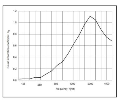
Mounting: The 11 panels were laid out flat on the concrete floor in the reverberation test room.
