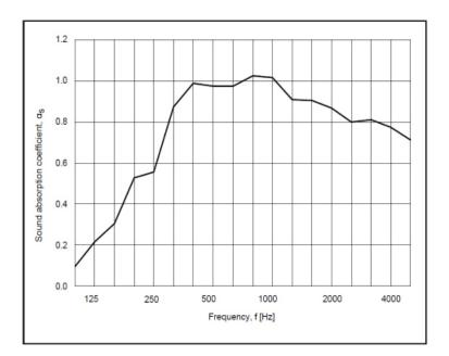
Mounting: Spacing 45mm behind panels. Closed frame around edges. Test Area 10.8 m2 Room volume 215 m2 Room surface area 305 m3
