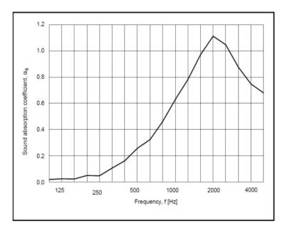
Mounting: The 11 panels were laid out flat on the concrete floor in the reverberation test room. Closed frame around edges. Test Area 10.8 m2 Room volume 215 m2 Room surface area 305 m3
