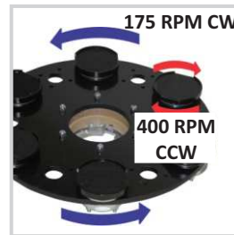
Driver Rotates at 175 RPM Tools Counter-Rotate at 600 RPM
