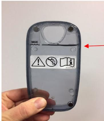
Reservoir should be filled to the 'Max Fill' line.
