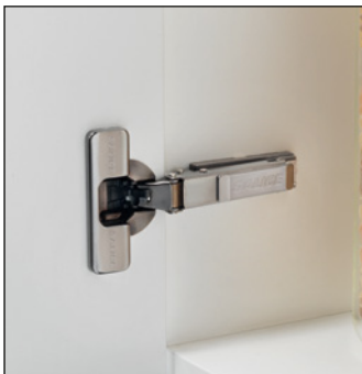
Silentia+ 200 Series Cup depth 15.5 mm and 13.5 mm Series for thick doors or 0 protrusion, 94° and 155° opening
