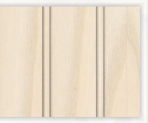
Columbia's Beaded Panels feature a wide variety of decorative hardwood faces and backs machined with a 11/2" or 3" on-center beaded groove pattern. The cutting heads are calibrated to ensure pattern uniformity across the entire sheet for a convincing illusion of tongue and groove woodwork that matches any existing species used. And since Beaded Panels are unfinished, close color matching with existing molding and millwork is possible. You can finish them or use them in painted applications.
