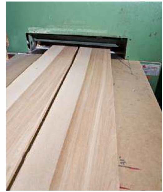
The flitch "books" are reviewed and graded to determine the best yield and quality and all sequences are kept together. Once this is complete the books are cut-to-length.
