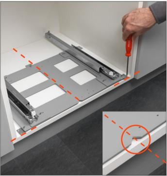
Pre-drill the drawer frontal using the template provided. For the correct positioning use as reference the middle of the front panel and its overlay  $(\mathbf{D})$  on the base panel of the cabinet.
