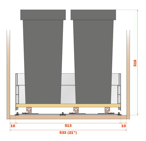
Position the runner support at the centre of the cabinet, using the front reference.
