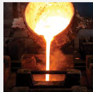
casting the escutcheon plate
