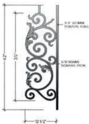
TOP VIEW A-3 ALL RADIUS FROM 28" TO 20"-Ø HFBX.A3
