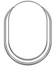
C-7237 4\text{-}\frac{5}{16}'' \times 6\text{-}\frac{3}{16}'' \times \frac{3}{4}'' Top panel width 3\text{-}\frac{1}{2}''
