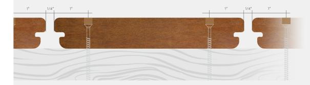
If you prefer the positive lateral connection of fastening through the face and still want a smooth, uniform surface, then using the Pro Plug® System with Kebony wood plugs is the best option. The Pro Plug® System by Starborn® is the fastest plug option on the market today, and Kebony wood plugs are designed to work seamlessly with the system.
