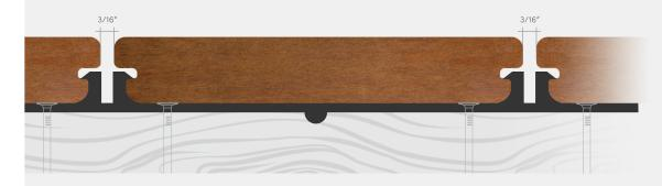
Step-Clip<sup>TM</sup> for Kebony uses easy to install strips to minimize the time and labor spent fastening your deck. The Step-Clip reduces deck surface installation time by up to 50% and ensures proper spacing, protects the joist from water damage, and makes it easy to replace a board in the future if necessary.
