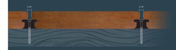
Hidden fastener clips are a great way to secure your deck without screwing into the board's face. Our Kebony Deck Board is compatible with the Fastenator™ Hidden Fastening system by DuraLife®.
