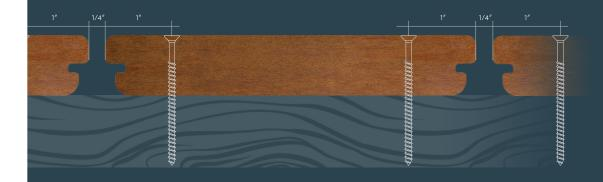
When securing your surface decking using traditional methods, you can use stainless steel screws through the face of our Kebony Deck Board. We recommend placing the screws 1" from the edge of the board.
