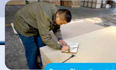
**Dragon Ply** quality control makes regular inspections of all process in the production cycle, including raw materials, press parameters, moisture content, bond, grade and thickness tolerance.
