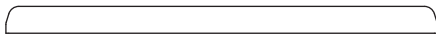
A 2 1/4" (57) width profile is available for most units to simulate a meeting rail or a multi-unit combination, such as a transom over a window or patio door.
