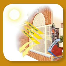
Low-E glass has a secondary, very thin metallic dual layer coating. This allows the sun's heat and light to pass through the insulating glass, but, at the same time, actually works to reflect radiant heat back toward its source. Since Low-E coating reflects radiant heat waves, it helps keep your home warmer in the winter by trapping radiant heat and cooler in the summer by blocking it from your home.
