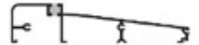
Standard Inswing Sill Thermally broken - 5-5/8" width. Optional extenders for larger wall sizes.
